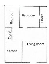
Scale: 1 inch on scale drawing corresponds to 12 feet in the actual apartment
